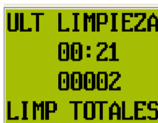
Photo: screen for most recent backwash & total no. backwashes.
